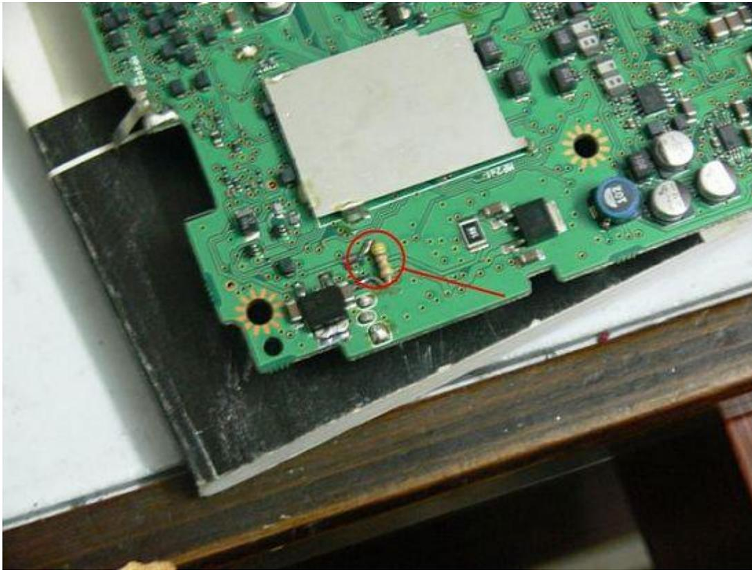
Tips: The click click problem can be caused by many other reasons but mainly if the contacts between radio and control head is loose, or there is a lack of power in any 5V or 8V line. For my case it was a burnt resistor caused by a short capacitor. Please check the followings in your radio:
