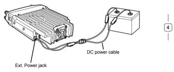
optional QCC-01(For Cigar-Plug connection) cable. Connect one of the cables between the ACC terminal or a Cigar-Plug that operates with the vehicle ignition or ACC switch on the vehicle and EXT POWER jack on the rear side of the unit.
