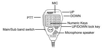
You can operate the transceiver by keypad or input desired frequency and channel through the QHM-05 microphone.
