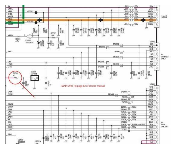
Ok, it looks like something else is shortening the output of that 7808. Traced the line and found it supplies power to the Display module (control head). One 7805 is there, checked and found ok. After checking all the capacitors found one of the big cap C502 is faulty. It is short. Removed it, checked everything else again.
