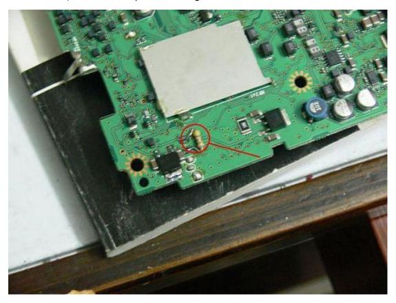
Tips: The click click problem can be caused by many other reasons but mainly if the contacts between radio and control head is lose, or there is a lack of power in any 5V or 8V line. For my case it was a burnt resistor caused by a short capacitor. Please check the followings in your radio:
