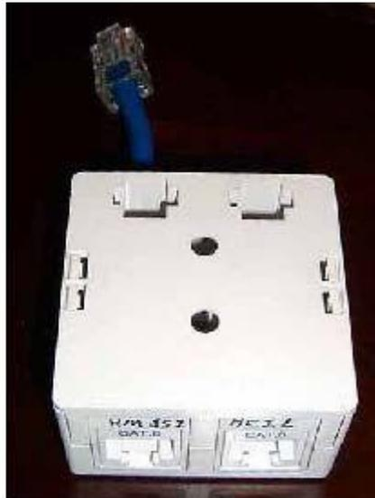
Each line represents a wire. Using the 2 port surface mount RJ45 jack allows you to just push down the wires without having to strip them first. Small caps come with the jack box too to keep the wires down.
