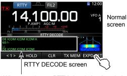
When tuned to an RTTY signal, the decoded characters are displayed.
