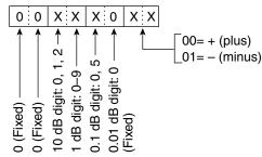
①Adjustable range:  $-20.0 \text{ dB} \sim +20.0 \text{ dB}$  in 0.5 dB steps
