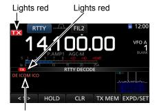
Contents being transmitted are displayed. (Example: transmitting the RT1's TX memory)
