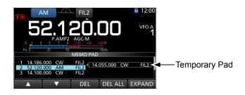
**TIP:** If you change the frequency or operating mode called up from Memo Pads, the contents are automatically updated in a temporary Pad.
