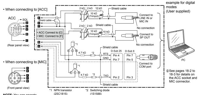
**NOTE**: You can operate ONLY AFSK RTTY when you connect the circuit to the microphone connector.
