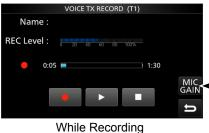
Touch to open the MIC GAIN adjustment window
