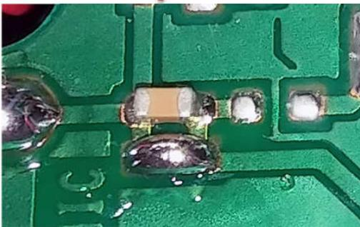
3 ---- With the help of a soldering iron remove the resistor, and shorting two pads with a drop of tin.
