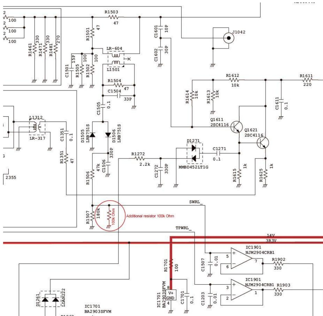
The best - experimentally found - value of the additional resistor is 100k Ohm. This value provides the practical matching range approx. SWR 1:6 (antenna impedance 8 to 300 ohm), that is much broader than originally.
