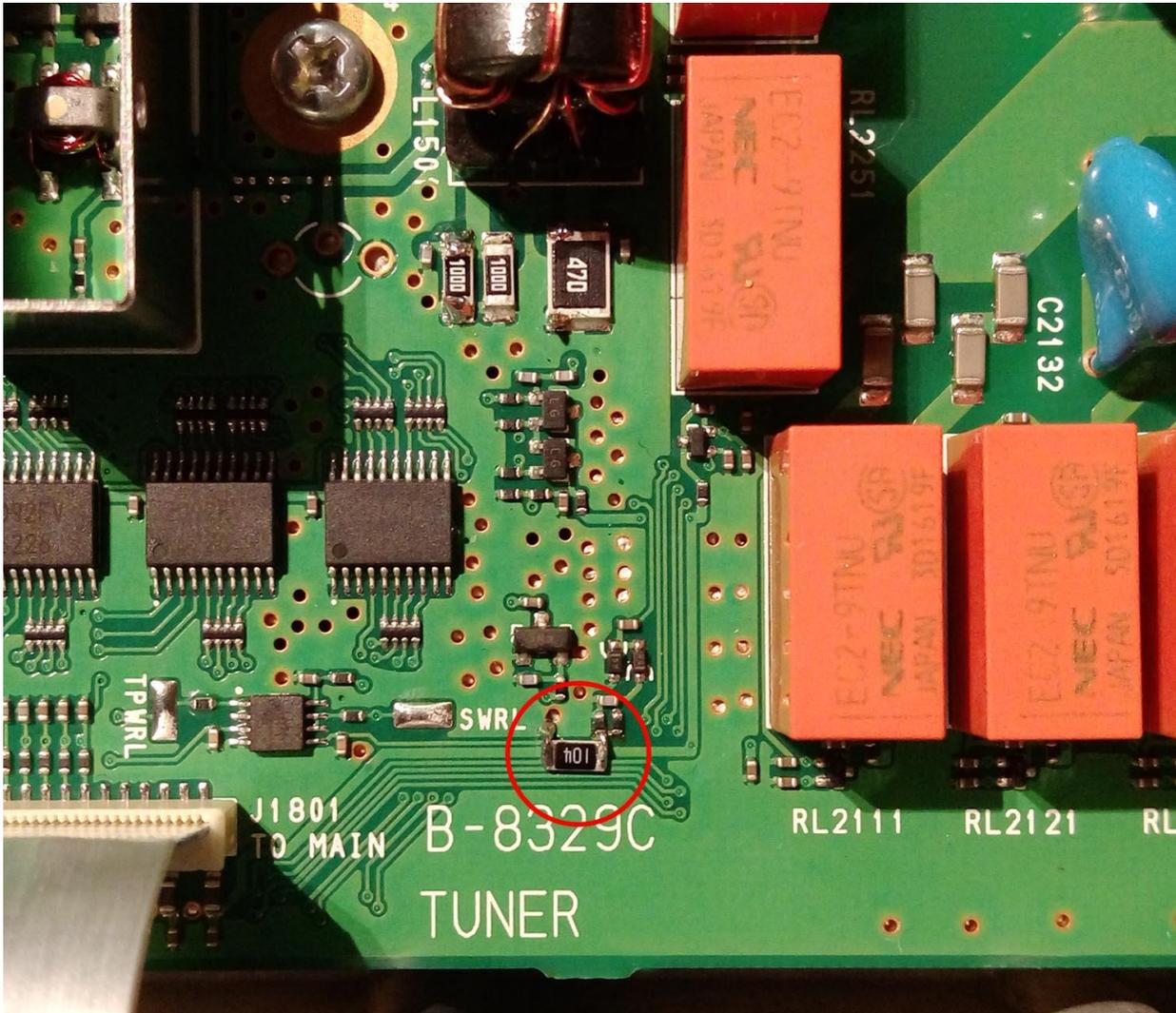
To do this mod, you have to remove the bottom cover of the radio and locate the resistor R1507 on the TUNER UNIT. It is above the "TUNER" inscription in the middle of the PCB. A soldering iron for SMD parts with a fine tip is needed to solder precisely to the resistor's lead. Take all the safety and EMC protection measures during the SMD soldering.
