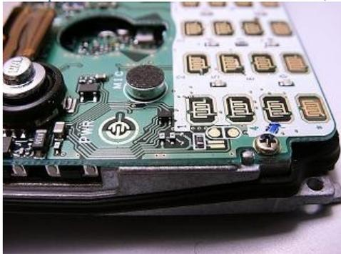
9. Remove only the top diode. There still should be two diodes in the middle and the bottom position.
