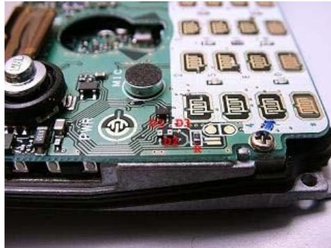
I will call these diodes D1, D2 and D3, starting from "Power" button, followed by the "R" (zero ohm) resistor.
