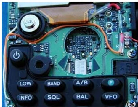
All you need is two pieces of thin wire and one small Reed switch. After the case is closed, entering the “Service Menu” is done using a small magnet (from about half inch distance).
