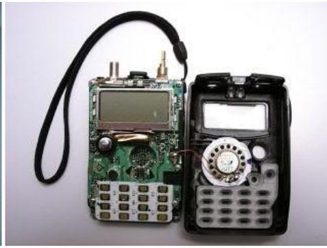
8. With the radio opened up like a book, look at the left hand side of the PCB just to the left of the PCB mounted microphone. You should see three diodes (if your transceiver is TH F6). In the next picture you will see only two diodes and an open pad, since the picture is from an TH F7E.
